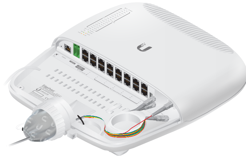
EP-S16 Strain Relief for Fiber Optic Strands
