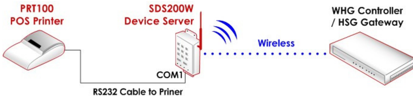
Diagram of SDS200W Connecting to PRT100 and WHG Controller wirelessly
